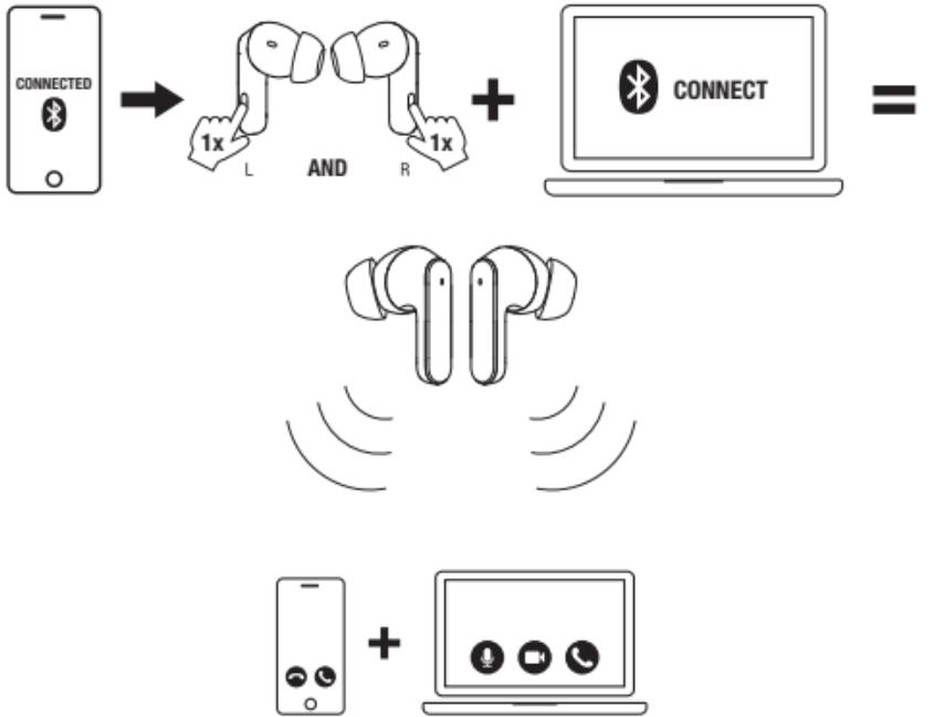
**EN** Multipoint connection: Press the left and right button simultaneously to pair and connect a second device. You can switch playback between devices. Only one audio stream is active at the same time. Voice assistant is active on the last paired device. Make sure music is not playing while pairing devices.
