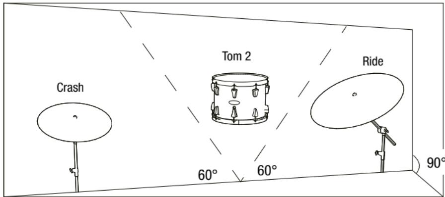
These are your drum positions. The LED indicator colour changes for each position. Red is the critical point. Do not strike in the red area, as your drumsticks are out of range there.
